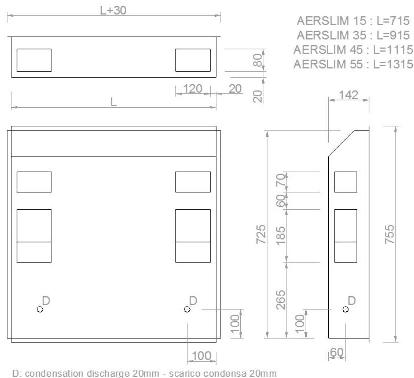
D: condensation discharge 20mm - scarico condensa 20mm
