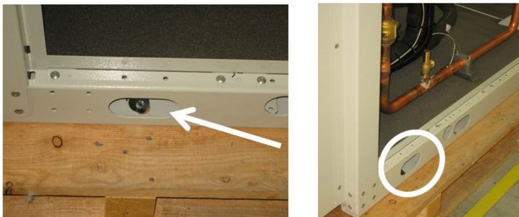
Fig. 10 Special positions of pallet fixing screws
